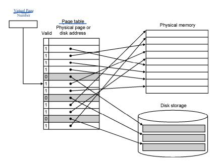
...is just a <u>mapping function</u> from virtual memory addresses to physical memory locations, which allows cacheing of virtual pages in physical memory.
