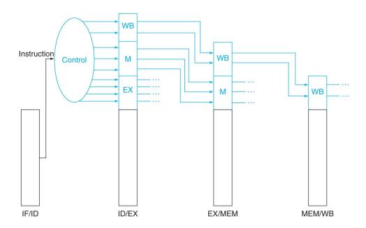
So, really it is combinational logic and some registers to propagate the signals to the right stage.
