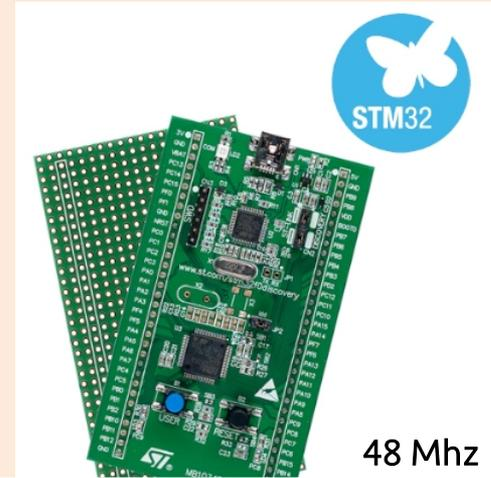
The Cortex-M0 processor is built on a highly area and power optimized 32-bit processor core, with a 3-stage pipeline von Neumann architecture. The processor delivers exceptional energy efficiency through a small but powerful instruction set and extensively optimized design, providing high-end processing hardware including a single-cycle multiplier.
