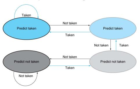
This state machine also referred to as a <u>saturating counter</u>. It counts down (on <u>not takens</u>) to 00 or up (on <u>takens</u>) to 11, but does not wrap around.
