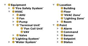
Figure 3: A subset of the Brick class hierarchy
