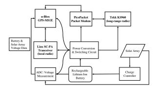
Figure 5: Block diagram of ZebraNet node design.
