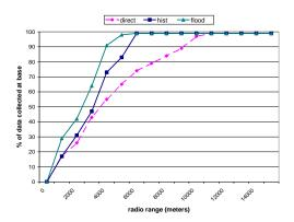
Figure 10: Success rate with infinite storage and bandwidth.
