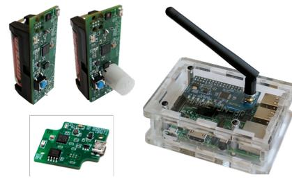
(a) WSN ecosystem: 1) with 6 sensors, 2) with 7 sensors (+PIR sensor), 3) small powered router, and 4) border router with a raspberry pi
