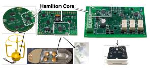
(b) Extended ecosystem: 1) ultrasonic anemometer, 2) auto-heating/cooling insole and smart desk fan (both with an actuator), and 3) thermostat
