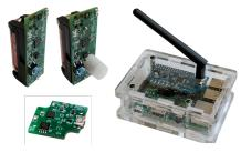
(a) WSN ecosystem: 1) with 6 sensors, 2) with 7 sensors (+PIR sensor), 3) small powered router, and 4) border router with a raspberry pi
