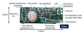
Figure 1: Hamilton, a single board that has a low-power 32-bit SoC and provides 7 types of sensors.
