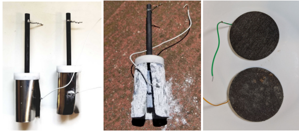
(a) Initial Zn-C cells. (b) Used Zn-C cell. (c) Used C-C cell.
