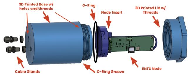
Figure 6: Exploded view of 3D printed enclosure
