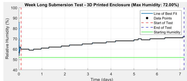
**(a) Humidity tracking over the 3D printed enclosure after a 7 day field test**
