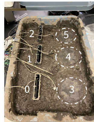
(c) Cells 0-2 are the new v3.1 cells while cells 3-5 are the v0 control cells. The same configuration was used for the v2 and v3 cells in Section 3.
